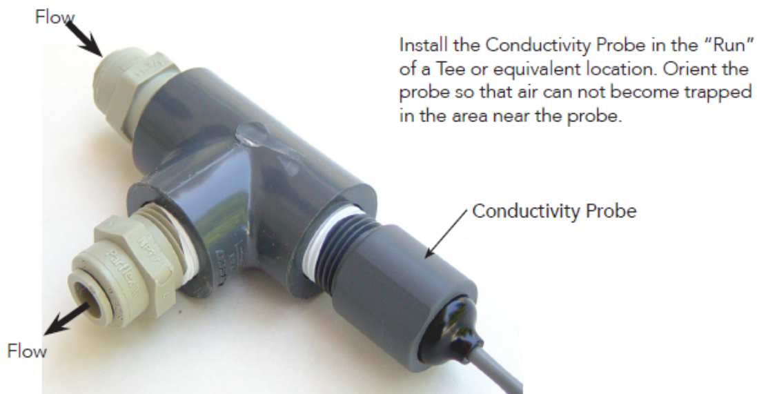
Figure 5. Conductivity Probe Installation
