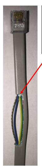
Strip back the Insulations to gain access to the bare drain wire and the blue wire.
