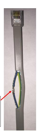
Or connect the 2 wires with a butt connector
