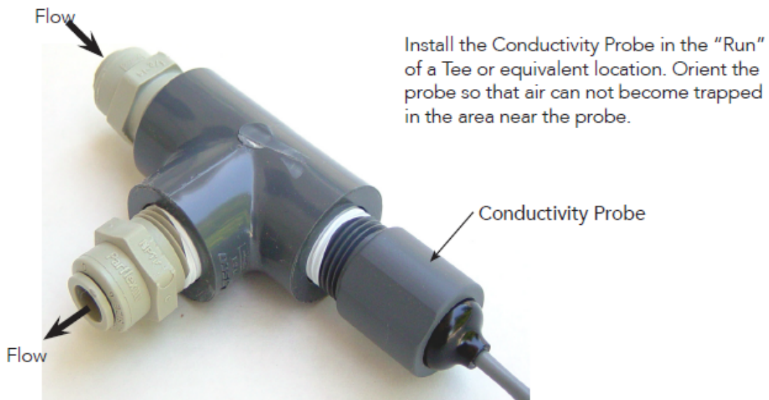
Figure 5. Conductivity Probe Installation
