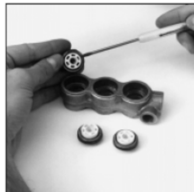
Installation of V-Packings
