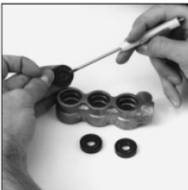
Installation of Lo-Pressure Seals
