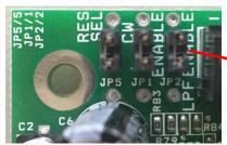
Move the Bimini jumpers away from cap to make it easier to access
