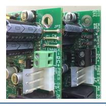
Main change is the Bimini Jumpers (Top Left). Now JP5 is label "RES SEL "it is used to select Marine air 10K ohms sensors or CA 3K ohms sensors.
