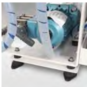
Vibration-isolation mounts reduce noise and vibration.
