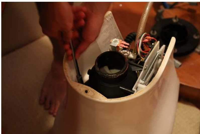
Remove main assembly – note 7/16in deep well socket
