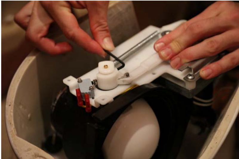
Tighten rotor shaft cam hex nut
