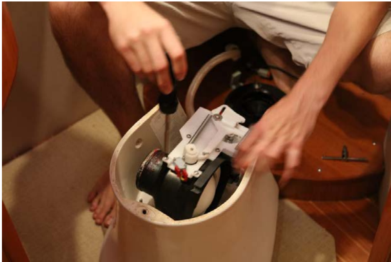
Place sideways to allow access to drive-arm and undo four mounting screws
