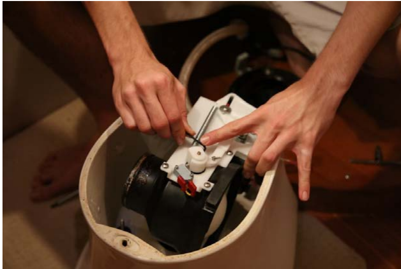
Loosen hex nut on rotor shaft cam (honestly who comes up with the names of these things)
