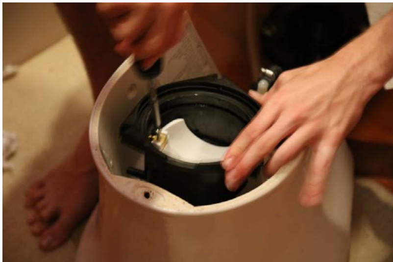
Rotate to gain access to locking screw
