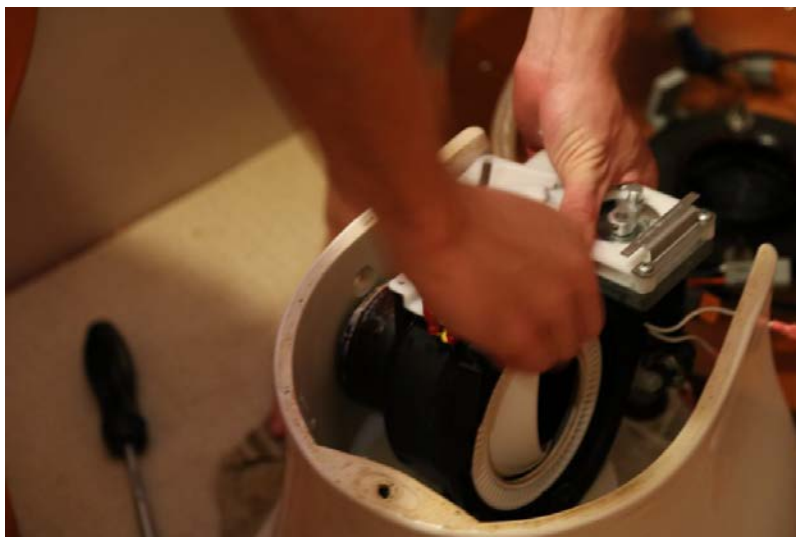
Gently ease drive arm board from main assembly
