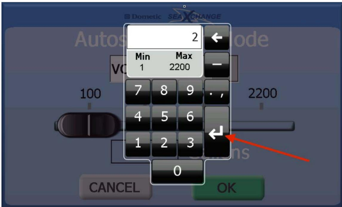
11. When (b) Volume is selected, there will be a sliding scale to select the volume of water the system will produce. Or touch the gallons/liters box and manually type in the volume, and press enter. Then press ok.
