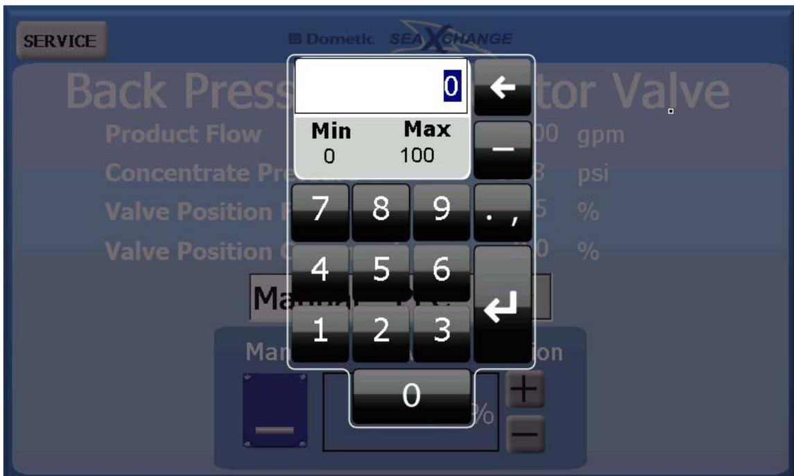
Manual – Hand will be displayed over the valve on the home screen, \*NOTE: After manual hand has been selected, the system will go into alarm when it is switched back to automatic. The alarm will have to be cleared to go back to normal operation.
