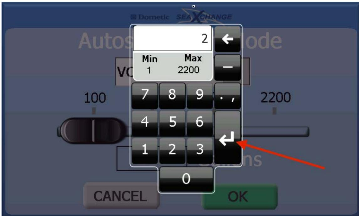
12. When the system is in auto shut down mode, there will be a count on the home screen that will track the production or the time of operation. When the system has satisfied the setting, it will shut down and do a fresh water flush.
