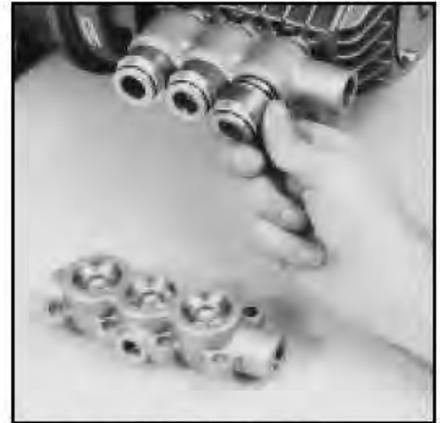
Removal of Adapter from Inlet Manifold
