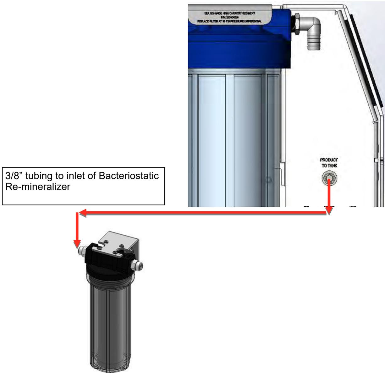
2. Run supplied white 3/8" tubing from filter assembly labeled **Bacteriostatic Re-Mineralizer** outlet to a dedicated fitting on or near the top of the ships fresh water tank. Be sure that there are no kinks in hose run and avoid 90's where possible to prevent restricted flow.
