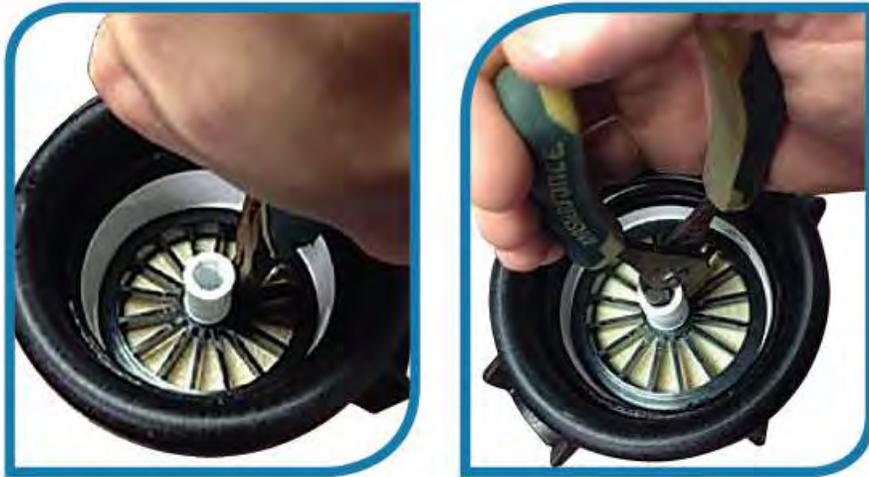
6. Remove new membrane element from container and inspect. Make sure that all parts are clean and free from dirt. Examine the brine seal, and permeate tube for nicks or cuts. Replace the O-rings or brine seal if damaged.
