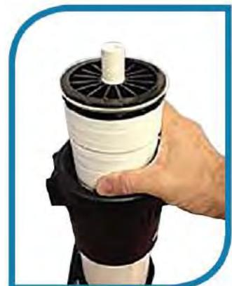
10. With a smooth and constant motion, push the membrane element into the housing so that the brine seal enters the housing without coming out of the brine seal groove. A slow twisting motion should be used to insert the membrane element, to ensure that the brine seal stays in place.
