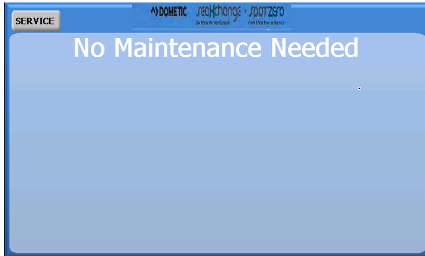
When maintenance is required a wrench and screwdriver symbol will appear at the top of the display. On the home screen this symbol can be pressed to bring up this screen. Perform the required maintenance then press reset.
