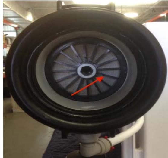
4. Slowly remove the membrane element from the pressure vessel being careful not to grasp it by the permeate tube. Needle nose pliers may be necessary to pull the old membrane element out of the pressure vessel.
