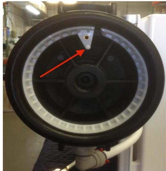
3. Remove the end cap from the pressure vessel.
