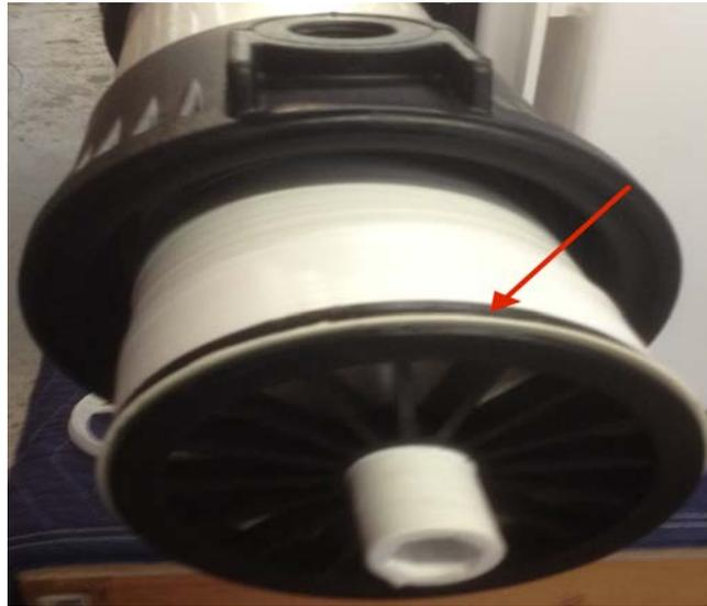
8. At a slight angle insert membrane element being careful not to tear or flip the brine seal. Re-lube the brine seal if necessary.
